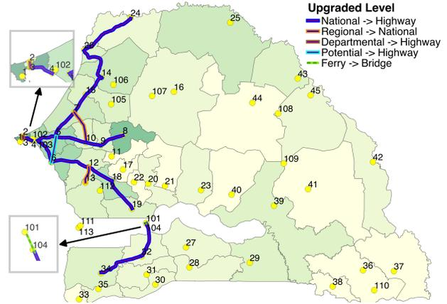
Figure 14: All Upgraded Links of the Optimal Solution to Achieve the Single Efficiency Objective
