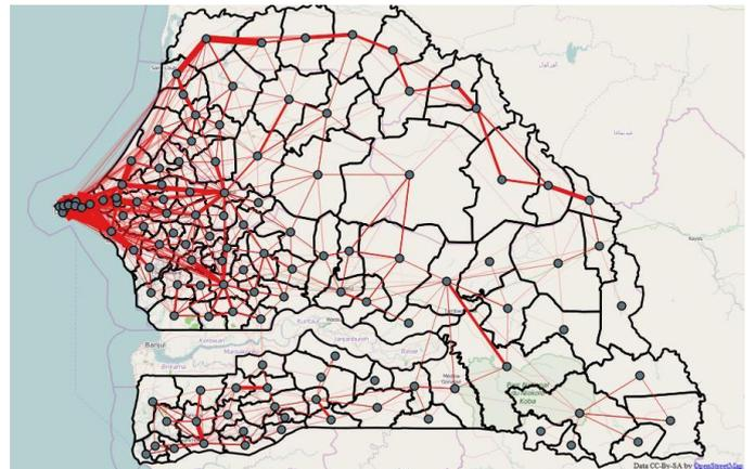
Figure 13: OD demand on the level of arrondissement for the first two week time period filtered on large OD demands.
