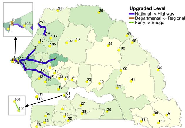
Figure 20: All Upgraded Links of the Optimal Solution to Achieve Efficiency Objective Given 1/2 Budget
