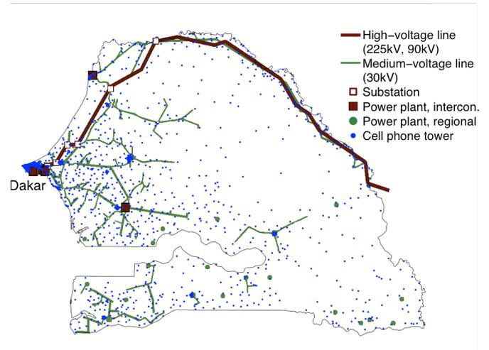
Fig. 1. Existing electricity infrastructure in Senegal and location of the mobile phone towers. The transmission and distribution network as well as the location of the power stations are adopted from [12].
