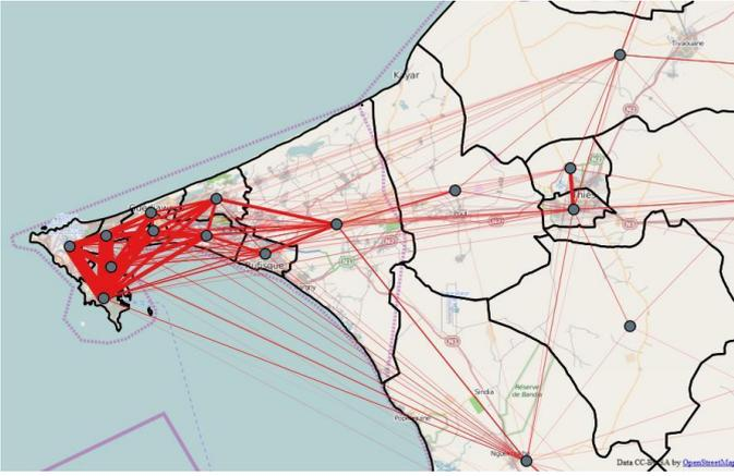
Figure 14: OD demand on the level of arrondissement for the first two week time period filtered on large OD demands for the Dakar area.
