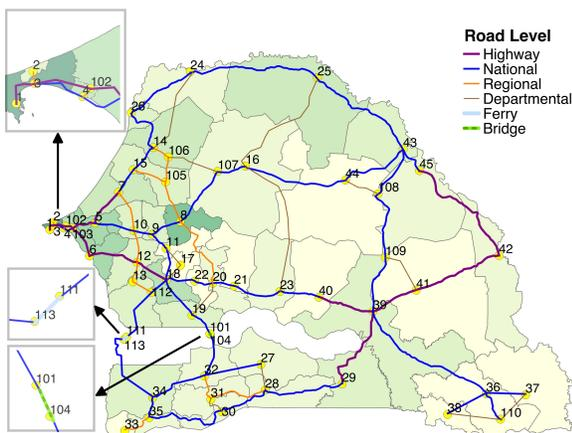
Figure 17: New Network of the Optimal Solution to Achieve both Efficiency and Equity Objective
