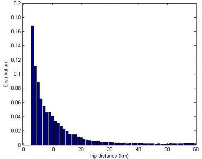
Figure 7: Trip distance distribution for the generated trips.
