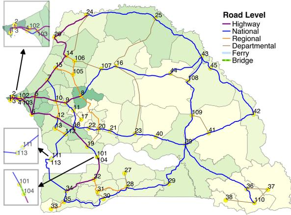
Figure 13: New Network of the Optimal Solution to Achieve the Single Efficiency Objective
