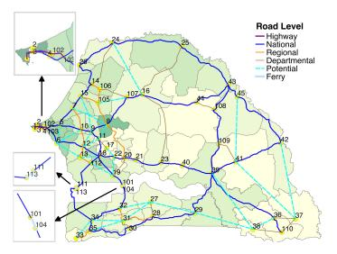
Figure 12: Potential Links to Be Added and Existing Links to Be Upgraded
