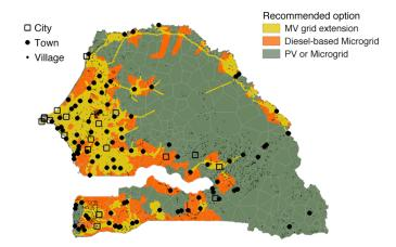
Fig. 7. Electrification recommendations considering 60% electrification levels and 13% migration to electrified villages.
