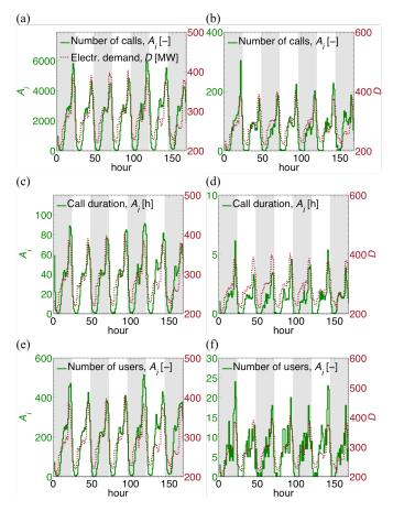
Fig. 4. Comparison of the mobile phone activity (measured as the hourly number of calls, call duration and number of users) with the aggregated electricity load profile (dotted line, in MW) for one week in January 2013 (Monday-Sunday). (a),(c),(e) Mobile phone tower in the city of Dakar. (b),(d),(f) Mobile phone tower in the rural area of Fayil. The shaded areas separate the different days.
