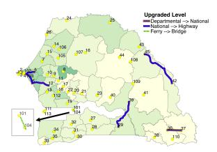
Figure 21: New Network of the Optimal Solution to Achieve Both Efficiency and Equity Objective Given 1/2 Budget
