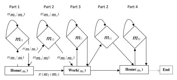
Fig. 3. The HMM for a home-based-work-tour
