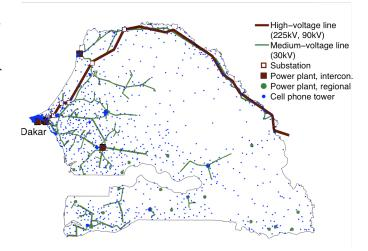
Fig. 1. Existing electricity infrastructure in Senegal and location of the mobile phone towers. The transmission and distribution network as well as the location of the power stations are adopted from [12].
